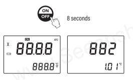
While continuing to hold the ON/OFF key, press the ZERO key. The temperature unit will change from °C to °F or vice versa.
