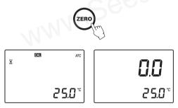
Gently absorb the ZERO water standard with a soft tissue. Use care not to scratch the prism surface. Dry the surface completely. The instrument is ready for sample measurement.
